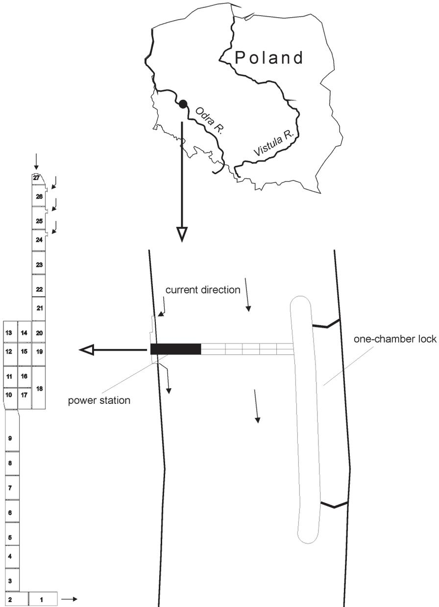
**Fig. 1.** Location of the dam “Waty Śląskie” and the scheme of the fish-pass. Small arrows indicate the water flow direction.
